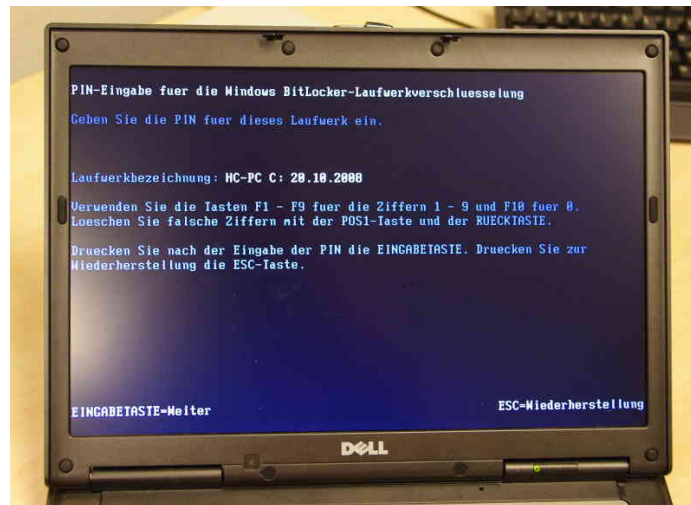
Fig. 1. Spoofed BitLocker PIN-entry screen.
